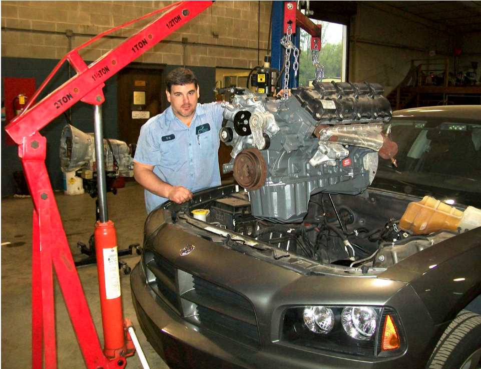
ESG's Team Opelika associate Eric Strong replacing the engine in a 2009 Dodge Charger for the City of Opelika Police Department.
